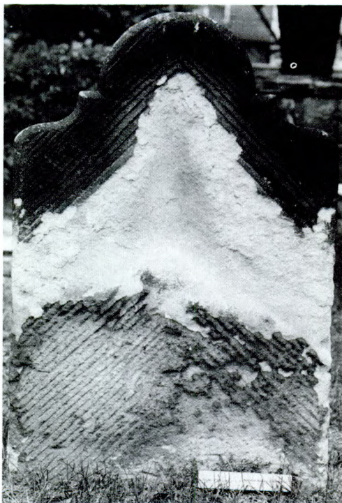
Surface crust on sandstone resulting from dissolution of the stone. Photograph: Erhard M. Winkler.
