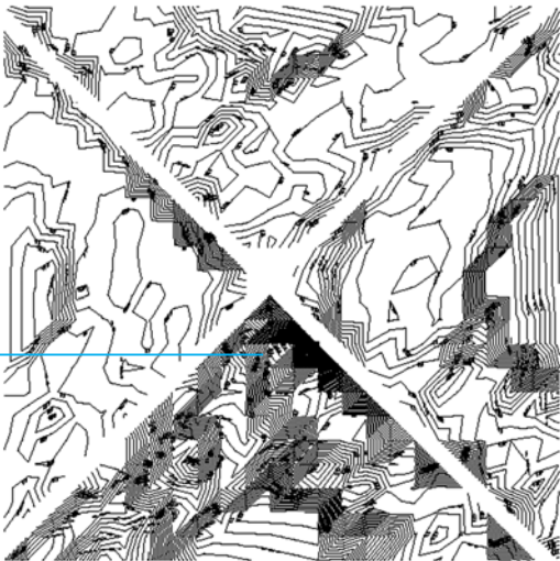
AREAS OF CONCENTRATED CONCENTRIC LINES AND DIMENSIONAL NOTATIONS IN THE PYRAMIDAL ROOF REPRESENT DEPRESSIONS INDICATING A LIKELIHOOD OF DETERIORATED FRAMING BENEATH THE SLATE.
